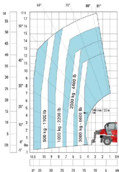
Machine on lowered stabilisers with forks Metric
